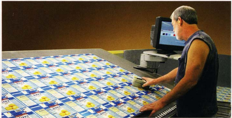
Don Whitney, second pressman, C&S Carton, uses X-Rite inspection equipment to check ink color densities produced by the KeyColor ink control system:
